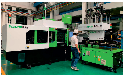
Fig. 17. The DCIM process allows compounding on the injection molding machine (© Yizumi)
