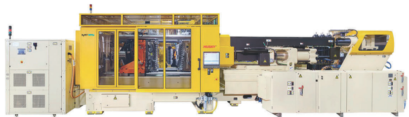
Fig. 9. The new HyPET HPP5e system permits the production of preforms with fewer rejects (© Husky)
