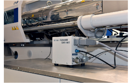
Fig. 8. The nitrogen for foam injection molding was collected from the ambient air (© Wittmann Battenfeld)
