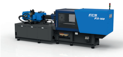
Fig. 6. The servohydraulic FCS FA-160 injection molding machine produces lunch boxes of PP at the K trade fair (© Windsor)
