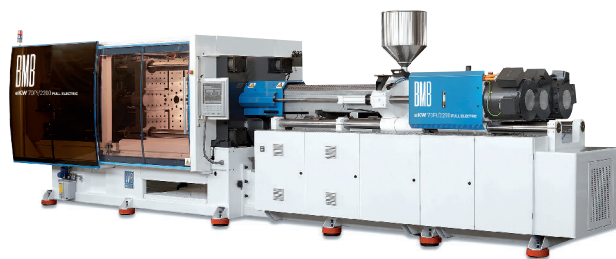
Fig. 11. The precision metering all-electric machine produces biodegradable coffee capsules with a micrometer-thin barrier layer (© BMB)
